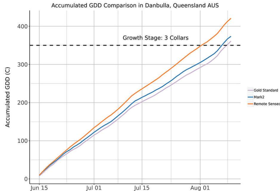
A 2020 comparison at an Arable Cal/Val site in corn in Australia co-located an Arable Mark 2 with a gold-standard weather instrument to compare infield growing degree days (GDD) against satellite-derived measurements. The study found that Arable's data resulted in GDD of about one day earlier than the gold-standard, and remote-sensed GDD were about seven days early.
