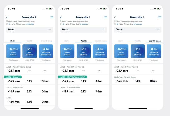
Select Water from the dropdown menu on the site details page to see water balance, soil moisture, Total Heat Stress Hours, irrigation runtime etc for this site. Water-in (precipitation/irrigation effective for crop growth), can be used for easy irrigation scheduling.
